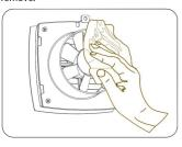
Clean the impeller blades. To remove dust use a soft brush, doth or a vacuum cleaner. Do not use water abrasive detergents, solvents, sharp objects. The impeller blades must be cleaned once in year.
